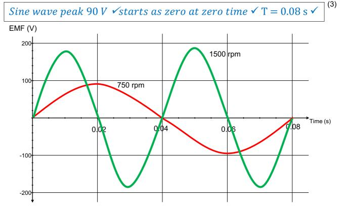
f) Sketch a second shape of the emf output for a rate of rotation of 1500 rpm and label this curve '1500 rpm'.
