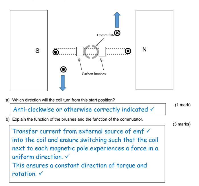
c) On the diagram above, use the symbols ● and ⊗ to sketch the location of the coil sides adjacent to the magnetic poles after 30° of rotation from this start position. Put arrows on your symbols to indicate the direction of magnetic force acting on them.
