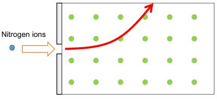
Vacuum chamber of mass spectrometer – magnetic field indicated
